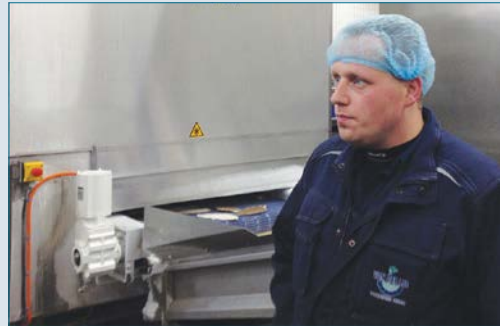
Willem Van der Lee (Van der Lee Seafish) standing near installed Bauer PMSM AsepticDrive.
